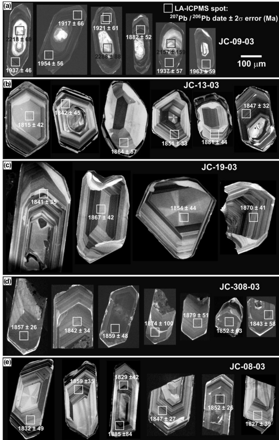
Fig. 5. CL images of zircon, showing location of LA-ICPMS spots with ^{207}\text{Pb}/^{206}\text{Pb} ages.
